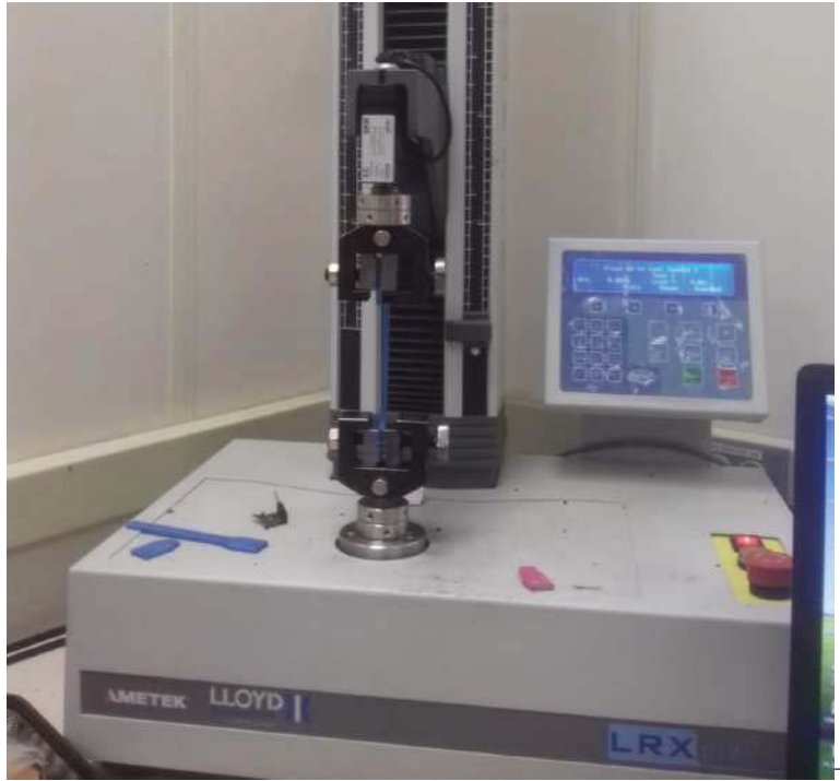
Figure 9: AMETEX load frame with 5 kN capacity.
